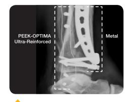
Radiolucent PEEK-OPTIMA Ultra-Reinforced polymer offers greater visibility than metal.
