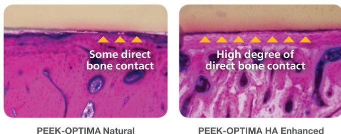
Figure 1: Cortical bone histology: Enhanced bone apposition at 12 weeks, greater direct bone contact with PEEK-OPTIMA HA Enhanced compared with PEEK-OPTIMA Natural.<sup>9</sup>
