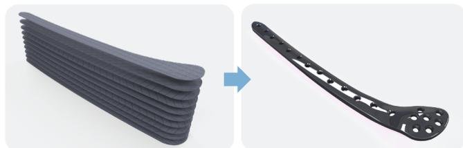
*Figure 1: Layers of carbon-fiber reinforced tape are the precursor to a fully finished fracture fixation component. This illustration is a simple schematic. Orientation of fibers and quantity of layers vary depending on application and mechanical requirements.*
